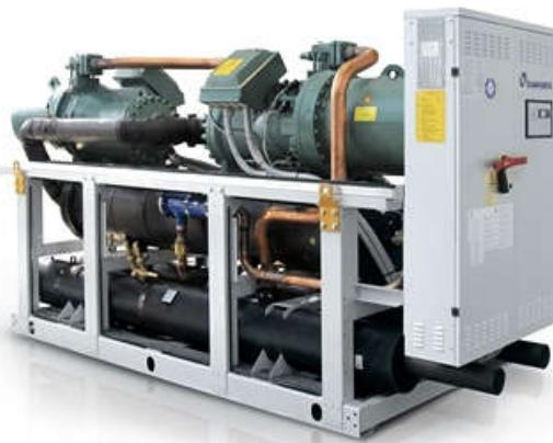
Unit for indoor installation for chilled water production. Semihermetic screw compressors optimized to operate with low compression ratio and R134a; shell and tubes condenser and direct expansion evaporator; electronic expansion valve. Frame in polyester-painted galvanized steel. High efficiency unit: the innovative optimized compressors and the high performing heat exchangers enhance EER values up to 5,1 (CA version) and even up to 5,6 (CA-E version) at Eurovent standards conditions.
