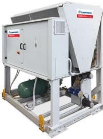
**Outdoor unit for the production of chilled water with semi-hermetic screw compressors optimized for R513A, axial-flow fans, micro-channel full-aluminum condensing coils, single-pass shell and tubes evaporator designed by Mitsubishi Electric Hydronics & IT Cooling Systems S.p.A. and electronic expansion valve.**
