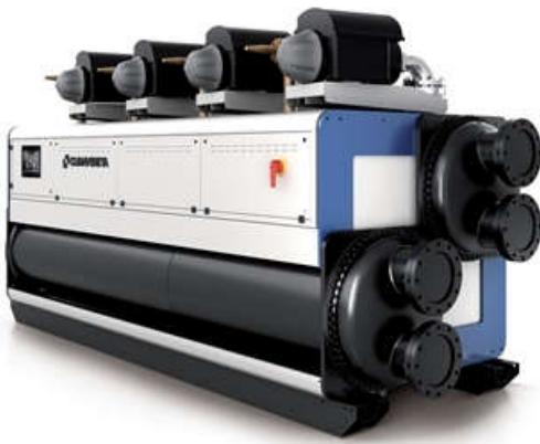
Indoor unit for the production of chilled water featuring centrifugal compressors oil-free, with R134a, electronic regulation valve, shell and tube condenser and shell and tube flooded evaporator.
