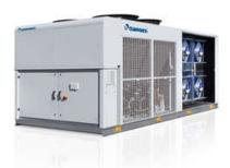
Autonomous reversible air-to-air Rooftop unit, for the thermo-hygrometric treatment, filtration and air renovation, in medium-large surface and volume ambient, such as supermarkets, shopping or exhibition centres. Hermetic rotary scroll compressors with R410A refrigerant; double refrigerant circuit fitted with Electronic Expansion Valves; EC plug fans are standard on these units.
