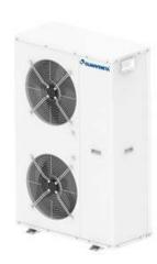
Outdoor unit for the production of chilled/hot water with variable speed (Inverter Driven) Scroll compressors, optimized for R410A in a single-circuit configuration, axial-flow fans, condensing coil with copper tubes and aluminum fins, plate heat exchanger on water side and electronic expansion valve as standard equipment.
